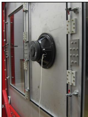
Speaker mounted on tunnel sidewall
