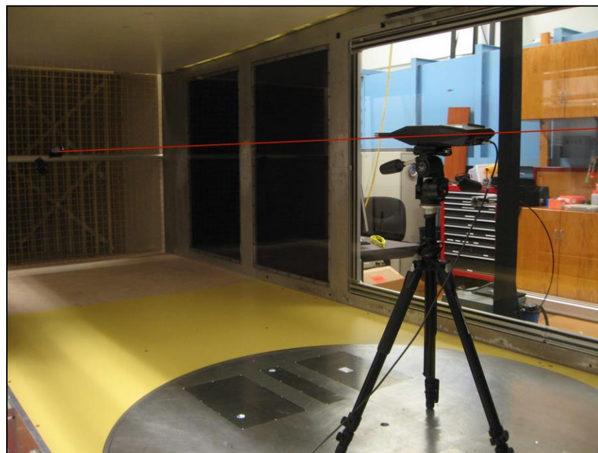
Microphone and laser beam path in the wind tunnel
