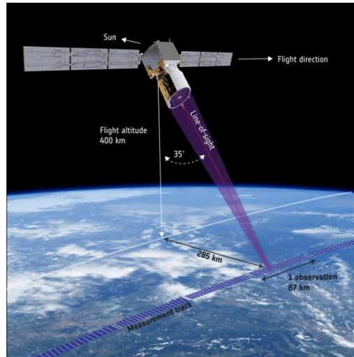
Figure 1. Aeolus orbit, pointing and sampling characteristics
