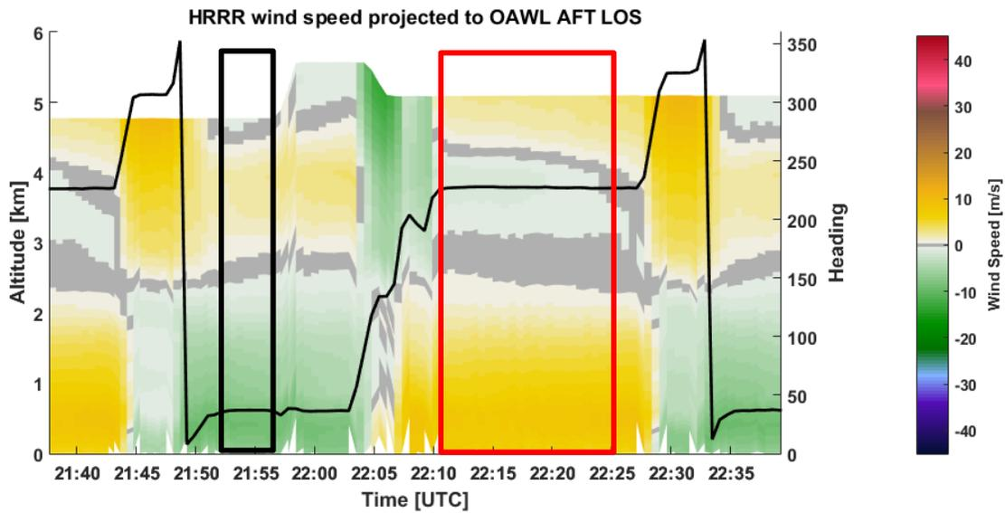
**Figure 3.** Projected LOS wind speed for OAWL AFT LOS using HRRR 0 hour forecast for 22 Z on May 10, 2016. The black line indicates the aircraft heading at the time of the OAWL data acquisition. The black and red boxes in the bottom panel indicate flight segment 1 and 2 respectively that is used for further analysis.
