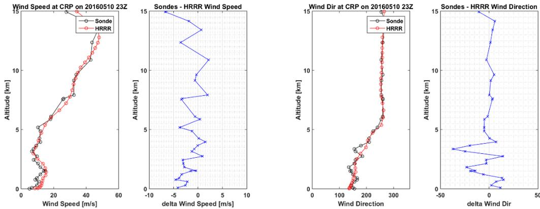
**Figure 5:** Comparison of wind speed (top) and direction (bottom) between Corpus Christi, TX 0Z radiosonde (launched at 23 Z) and HRRR 0 hour forecast for 23 Z at the radiosonde launch site on May 10, 2016. HRRR data were interpolated to the radiosonde altitude. The right panels show difference between the radiosonde and model data.
