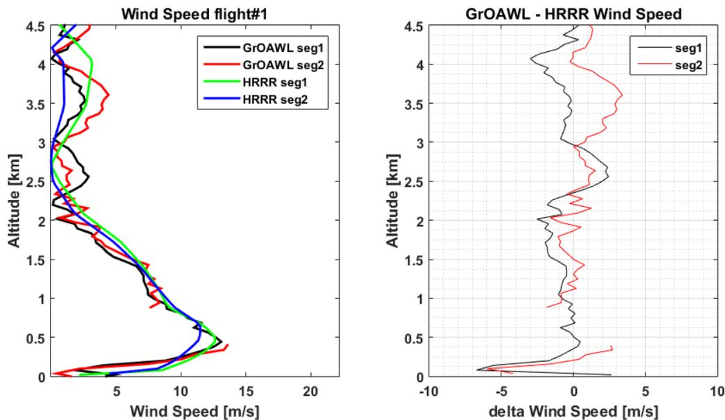
**Figure 4:** Mean horizontal projection of wind speed profile for OAWL (black and red) computed from AFT look at 355 nm only and HRRR (green and blue) for two flight segments at constant altitude and heading. The flight segments are marked by boxes in Figure 3. The right panel shows difference in wind speed between OAWL and HRRR for the two segments (Preliminary data).
