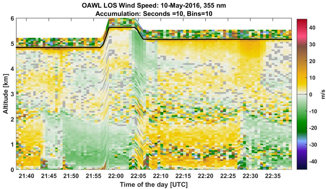
**Figure 2:** LOS wind speed measured by the AFT look of the OAWL instrument at 355 nm during flight #1 on May 10, 2016 (Preliminary data).
