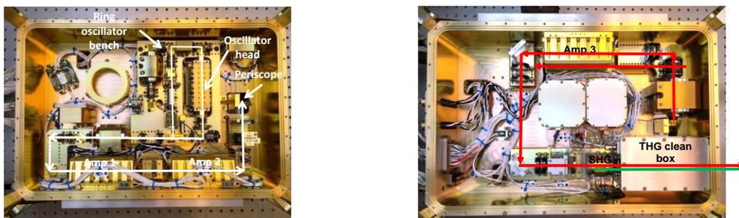
Figure 1. UVLD oscillator/pre-amplifier (l) and power amp/nonlinear converter(r) compartments
