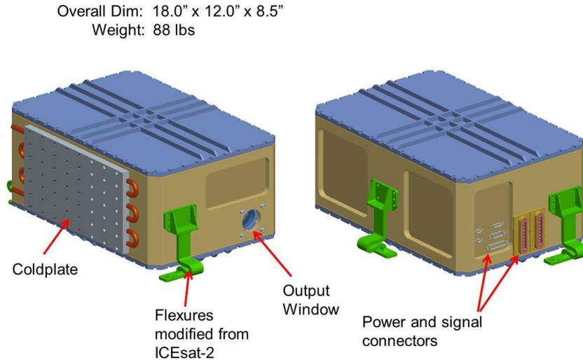
Figure 2. Dimensions, weights and interfaces of the UVLD laser optics module
