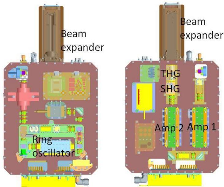
Figure 4. ATHENA OAWL oscillator (left) and amplifier (right) compartments
