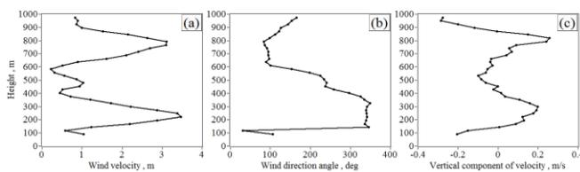
Figure 3. Vertical profiles of the wind speed (a), the wind direction angle (b), and the vertical component of the wind vector (c). Data of Fig.1 (measurement time 14:31 LT).
