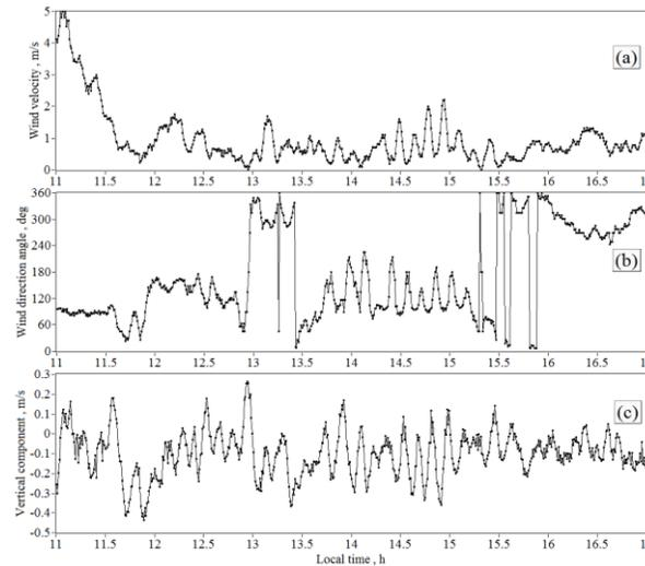
Figure 2. Temporal profiles of the wind speed (a), the wind direction angle (b), and the vertical component of the wind velocity (c). Data of Fig. 1 (measurement height of 636.5 m)
