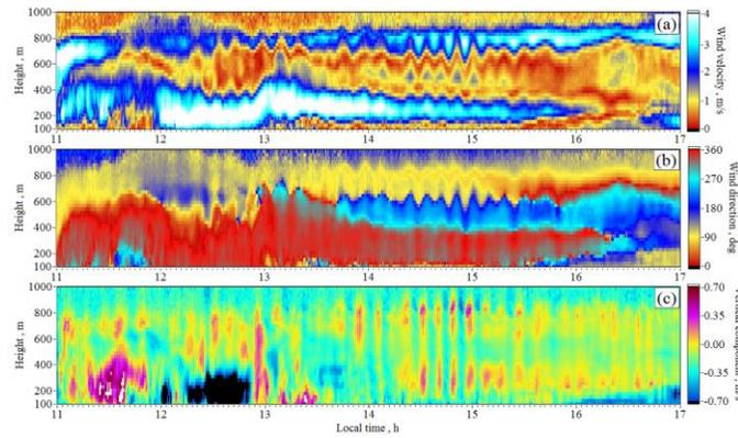
Figure 1. Spatiotemporal distributions of the wind speed (a), the wind direction angle (b), and the vertical component of the wind vector (c) obtained from measurements with the Stream Line lidar on August 23 of 2015. The height is given relatively to lidar position height.
