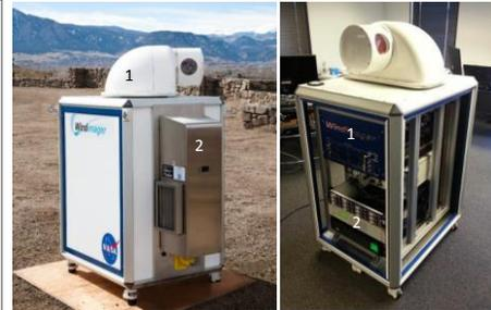
Figure 3. The Windimager™ lidar unit. Left Picture: (1).Hemispherical scanner, (2). Air cooled unit. Right Picture The internal arrangement. (1).The lidar transceiver chassis. (2). The UPS unit
