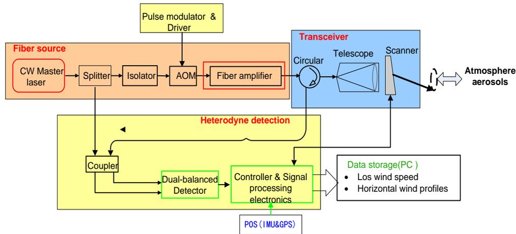
Figure 1. The block diagrams of the CDL system
