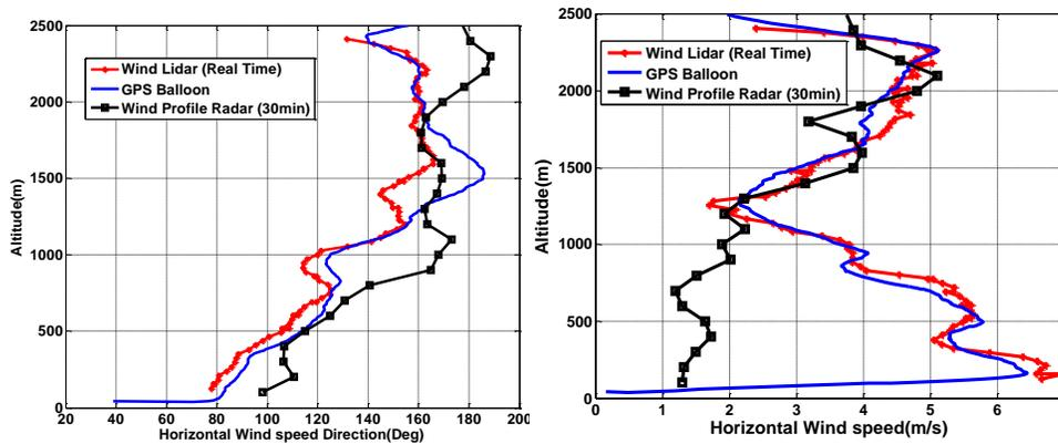
Figure 3. The comparison between the lidar, Radar, and the GPS sounding
