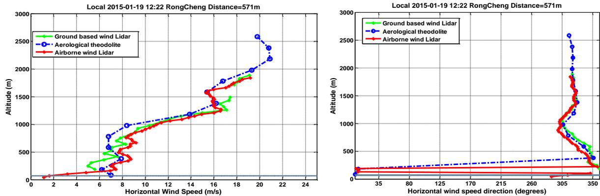
Figure 4. The wind speed profiles comparisons between the three systems.
