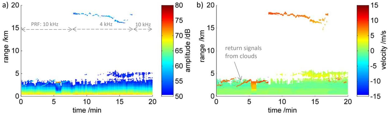
Figure 2. Measurement example of an ambiguity due to clouds.
