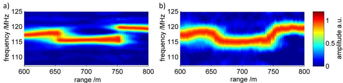
Figure 5. Measured wind shears in the frequency domain for different probing pulse lengths.
