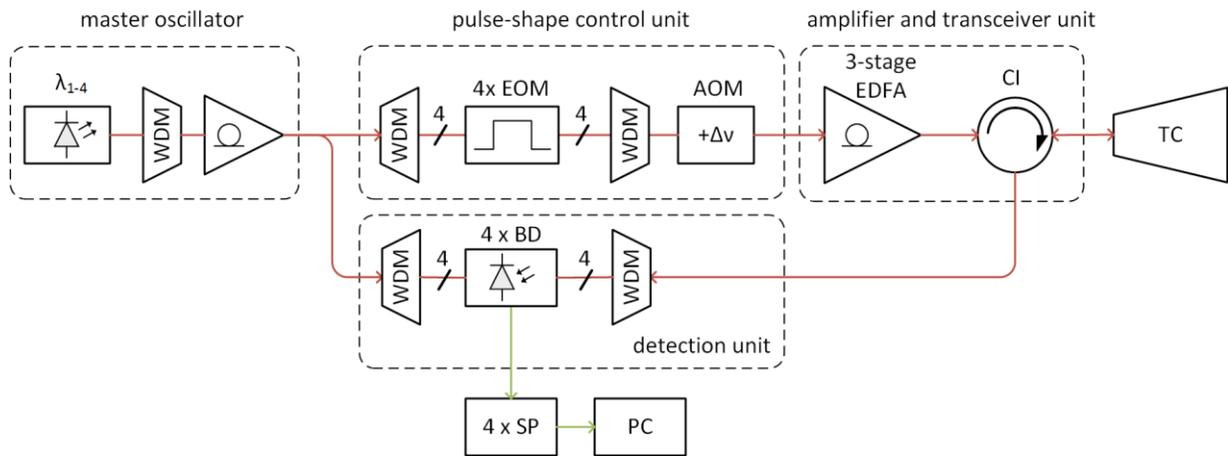
Figure 1. Overview of the multi-channel coherent Doppler lidar system.
