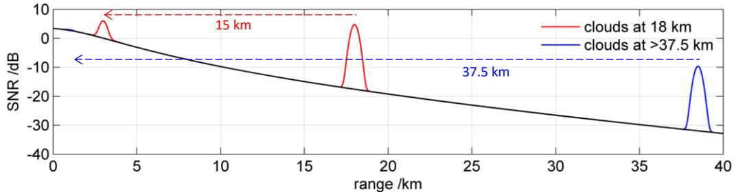
Figure 3. SNR as a function of range predicted by the lidar equation.
