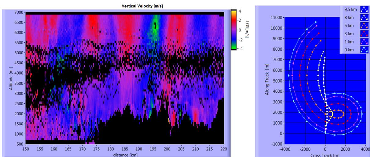
Figure 2: Example of vertical wind due to gravity waves (left) compared to the footprint of a conical scan
