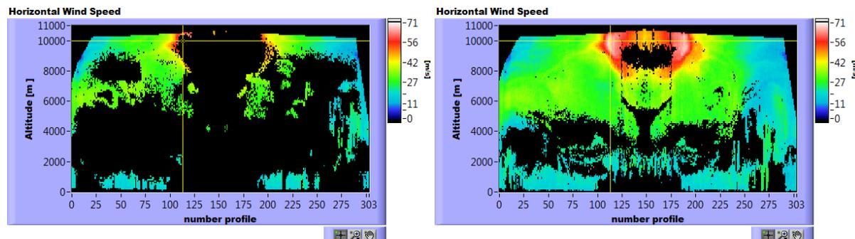
Figure 1: Example of increased coverage with the modified accumulation algorithm (right) compared to standard LOS inversion algorithm (left).
