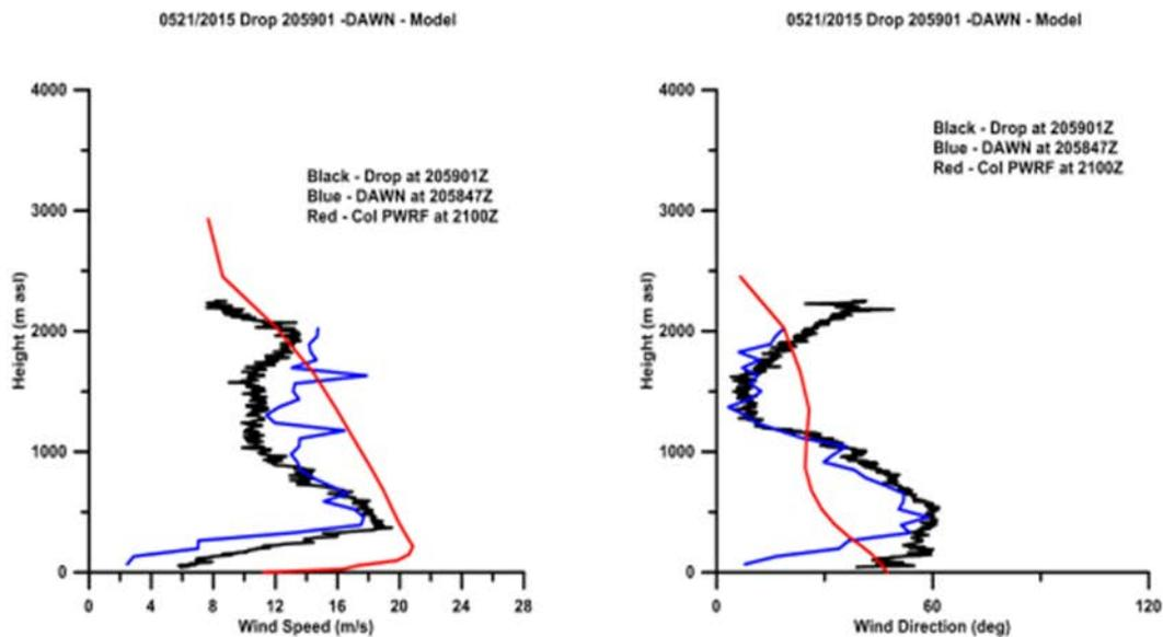
Figure 3. Wind speed and direction profiles for dropsonde (black), DAWN (blue) and Colorado Polar WRF (red) forecasts centered on the time and location of the 205901Z drop on 05/21/2015.
