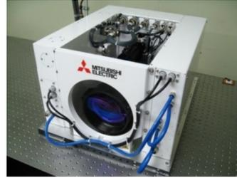
Figure 7. Optical Antenna of the Next Doppler Lidar.
