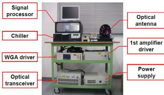
Figure 2. High Altitude Lidar Model.
