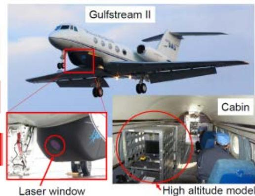
Figure 3. Experimental System Installation.
