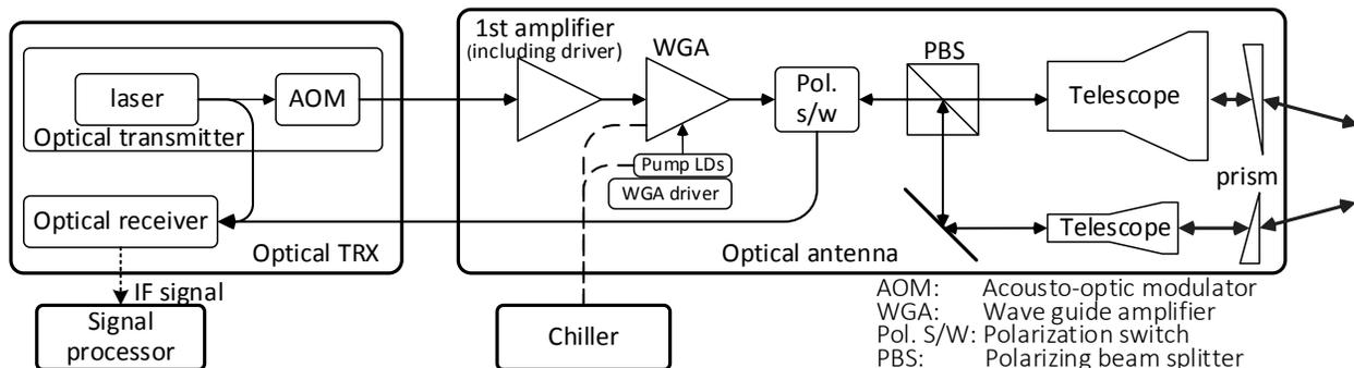
Figure 6. Schematic Diagram of the Next Doppler Lidar.
