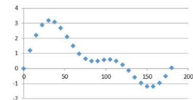
Figure 3a: Sum of 4 sine waves, 11, 7, 5, and 3 Mhz,
