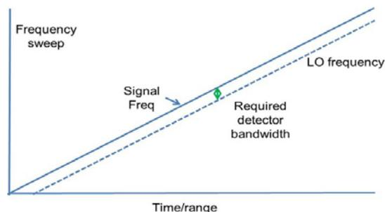
Figure 1: Stretch Processing Sweeps the LO and the transmitter in sync
