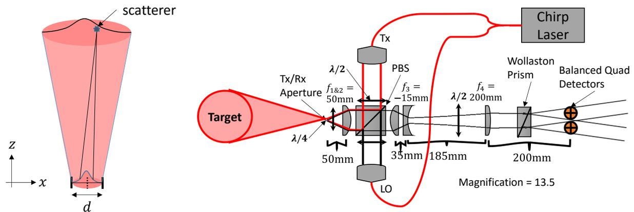
Figure 1. (Left) Differential SAL (DSAL) concept diagram. (Right) DSAL receiver design.
