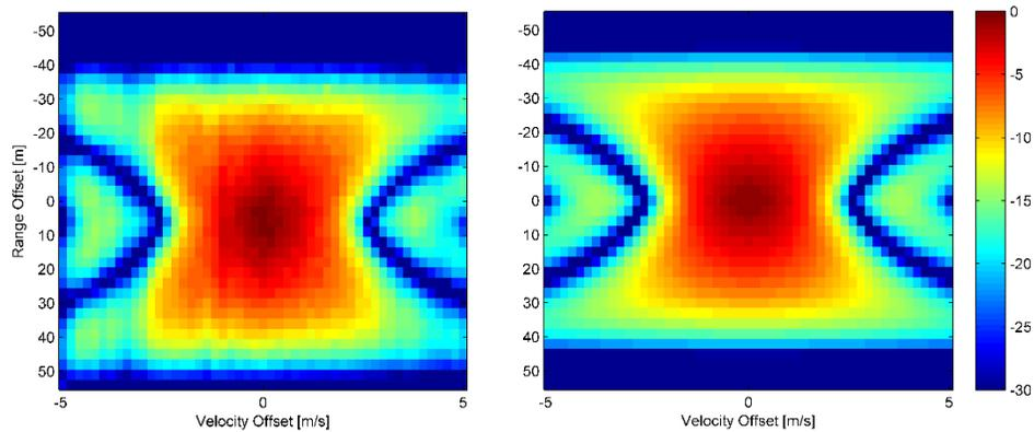
Figure 4. (left) Measured CNR vs. range and Doppler offset. (right) Theoretical CNR vs. range and Doppler offset obtained from Eq. (4). CNR is displayed in dBs.
