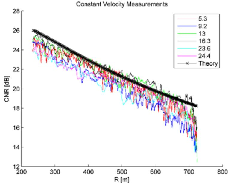
Figure 3. CNR vs. range for moving and non-moving target
