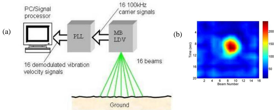
Figure 1. (a) Setup of scanning MB-LDV for acoustic landmine detection, (b) Vibration image of a buried landmine.
