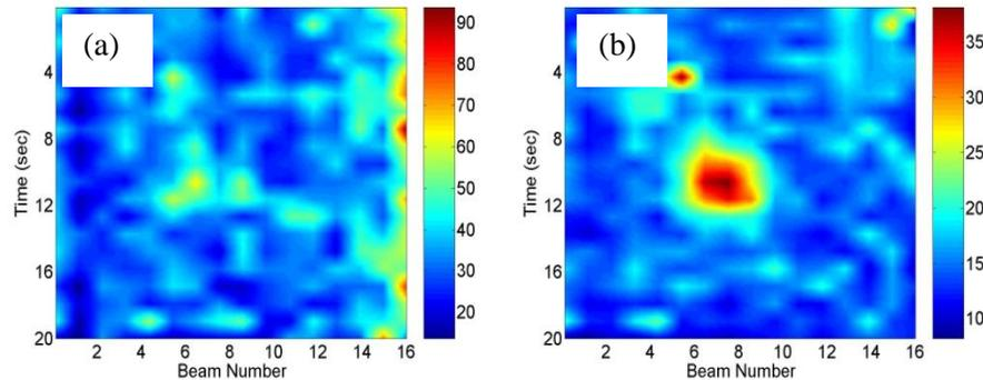
Figure 3. Velocity image of buried antitank mine before (a) and after (b) the wavelet threshold method of speckle noise reduction was applied.
