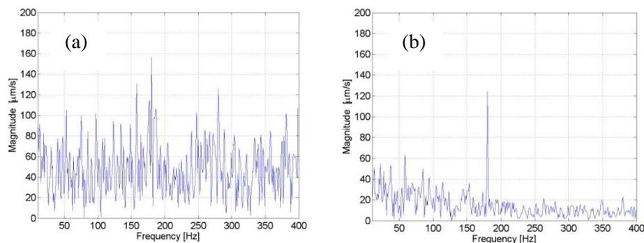
Figure 2. Spectrum of a continuously-scanning LDV velocity signal. (a) signal contains spikes; (b) spikes removed from the signal.
