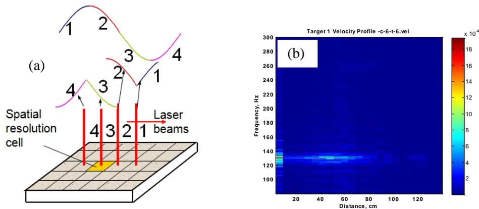
Figure 4. Principle of time-multiplexed laser vibrometry (a) and a vibration velocity profile of a buried plastic mine measured at 0.73 m/s speed.
