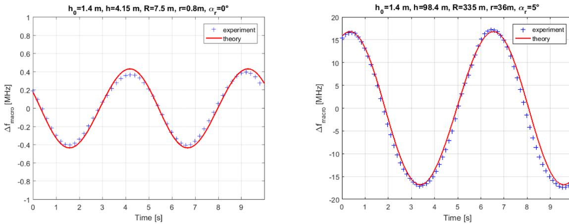
Figure 4. Theoretically estimated (red) and measured (blue) macro Doppler shifts for our wind turbine model (left) and the real wind turbine Vestas V90 (right) during 10 s time duration.
