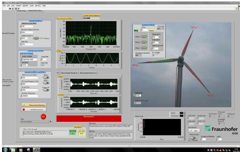
Figure 3. User interface with parameter settings, data acquisition, display and visualisation of the measurement points.
