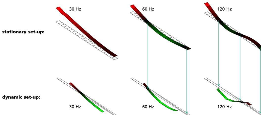
Figure 5. The first three blade vibrational modes of our wind turbine scale model (stationary and during rotation) measured with the laser Doppler vibrometer.
