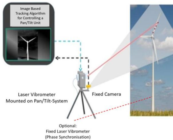
Figure 1. Principal system configuration.
