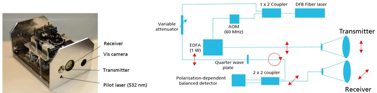
Figure 2. Experimental 1.5  $\mu\text{m}$  laser Doppler vibrometer using polarisation diversity.
