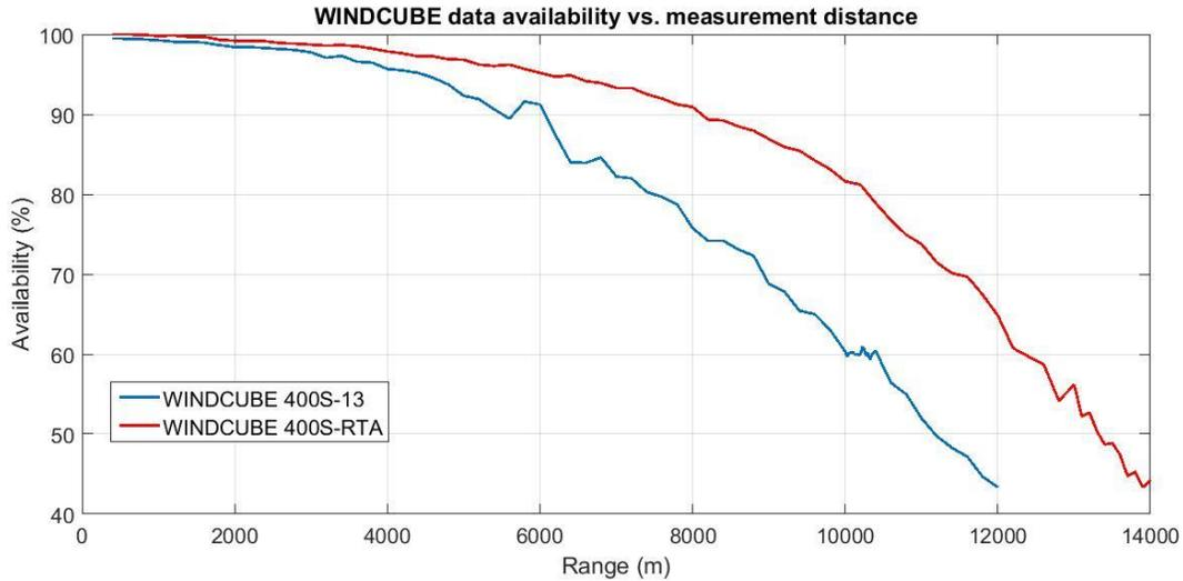
**Figure 3 WINDCUBE 400S-13 data availability vs. measurement distance for the entire data set**
