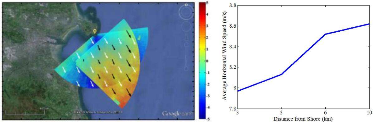
**Figure 5** Wind speed map over the area and wind speed variation with distance from the shore.
