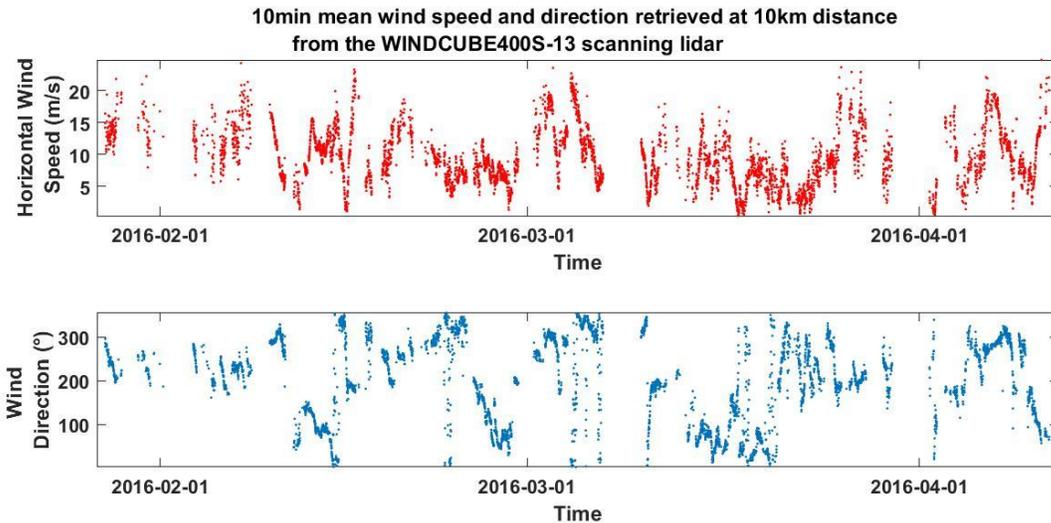
**Figure 4 WINDCUBE 400S-13 calculated 10min averaged wind speed and direction at 10km distance from the Lidar**
