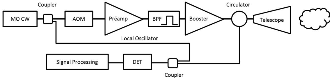
**Figure 1 Architecture of fibered pulsed lidars**
