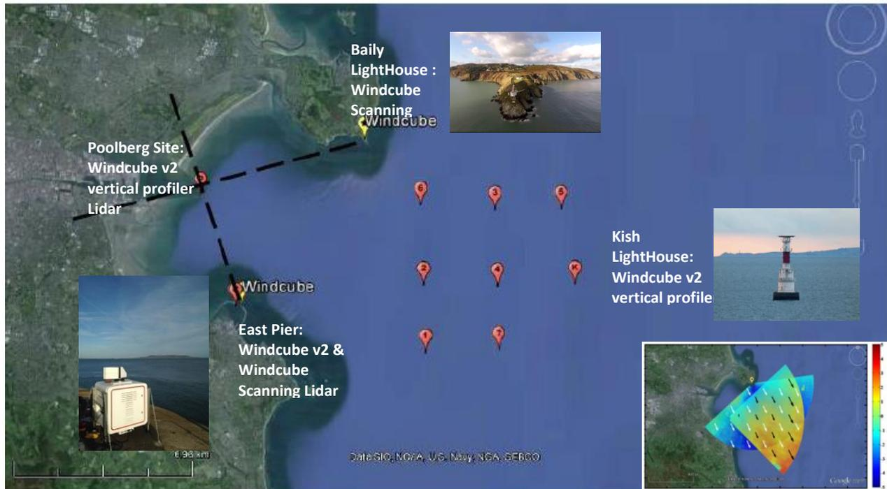
**Figure 2 Measurement campaign set-up with locations of Lidars**
