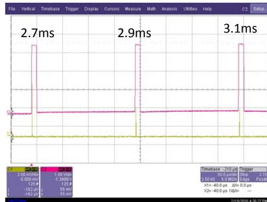
Figure 3. Oscilloscope record for the successful triple-pulse operation.
